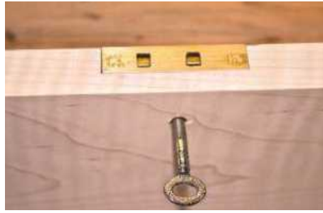
▲ Pic.11 I laid the back of the lock flat against the inside centre and top edge, marked it, routed it with a straight bit, followed by a small chisel to square the corners. The lock fit snugly
